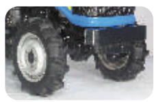
4WD FRONT AXLE (For better traction. Suitable for muddy operation better steering angle for sharp turning)
