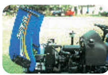
3 CYLINDER ENGINE (High torque fuel efficient low noise & vibration)
