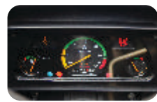
ELECTRONIC INSTRUMENT CLUSTER WITH BACKLIT (Easy to see at night)
