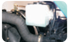
RADIATOR OVERFLOW RESERVOIR (No need to fill coolant again & again)
